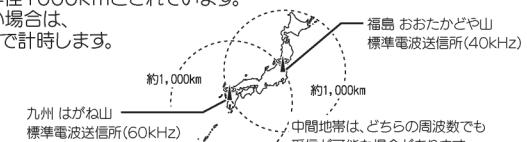
The diagram illustrates the coverage area of the standard radio wave signals. Two stations are shown: Haganeyama (standard radio wave signal at 60kHz) and Ootakadoya (standard radio wave signal at 40kHz). The coverage area is roughly circular with a radius of about 1,000 km. The map shows the locations of the stations and their respective coverage areas.
